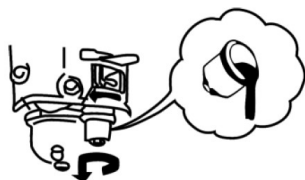
1. Turn the fuel tap to "OFF" position, remove the fuel filter cup, and drain off the fuel in the cup. (Model: Simple unit)
