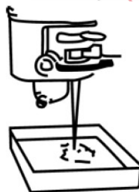
2. Unscrew the fuel valve and drain all the fuel. (Model: Simple unit)
